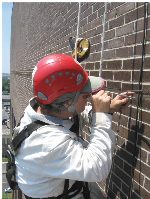
Mike Gilbert using a boreoscope at Dulles State Office Building in Watertown, NY
