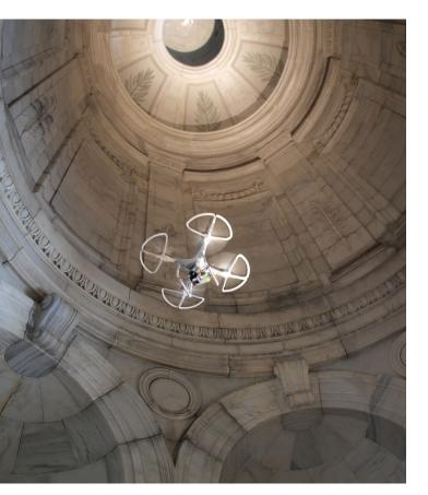
ertical Access operates a fleet of DJI<sup>™</sup> Phantom quadcopter Unmanned Aerial Vehices (UAVs, or drones) to aid in the investigation of buildings and infrastructure. Our team of FAA-certified UAV pilots utilize drone technology in a number of applications ranging from reconnaissance surveys highlighting areas of concern for further investigation to flying lightweight rigging cords up and over structural elements to gain hands-on access.
