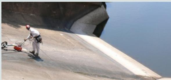
VA was retained by [Olson Engineering](#) to assist with nondestructive testing (NDT) at the Occoquan Dam in Fairfax County, Virginia in August. The purpose of the project was to perform an investigation of the dam's North abutment (side spillway) using Ground-Penetrating Radar (GPR) to determine the rebar size and spacing in this portion of the dam.
