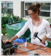
Our interest in the mock-up project was to construct portions of the vault with known faults (primarily delaminations between tile wythes). VA Partner Kelly Streecher has done some preliminary NDT testing using ultrasound to evaluate the structural integrity of multi-wythe tile vaults that has been promising. The MIT vault,
